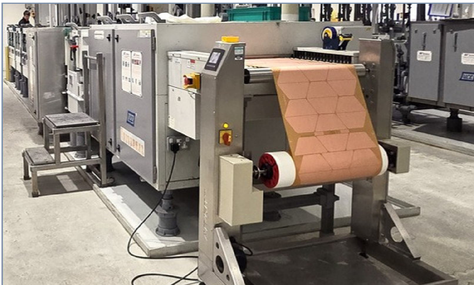
Long flex PCB manufacturing made possible with IHT
